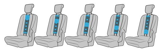
The fastening straps are used to buckle up the belt at the rear of the seat. Place the upper straps over the backrest, and pull the lower straps through the gap between the backrest and the seat. Next, buckle up and properly tighten the straps.
