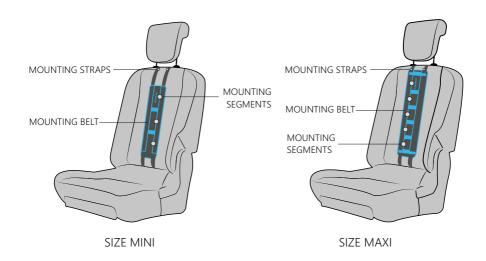
The loops in the fastening belt make it possible to install the other elements of the Belticar® System at the appropriate height, depending on the user's needs.
